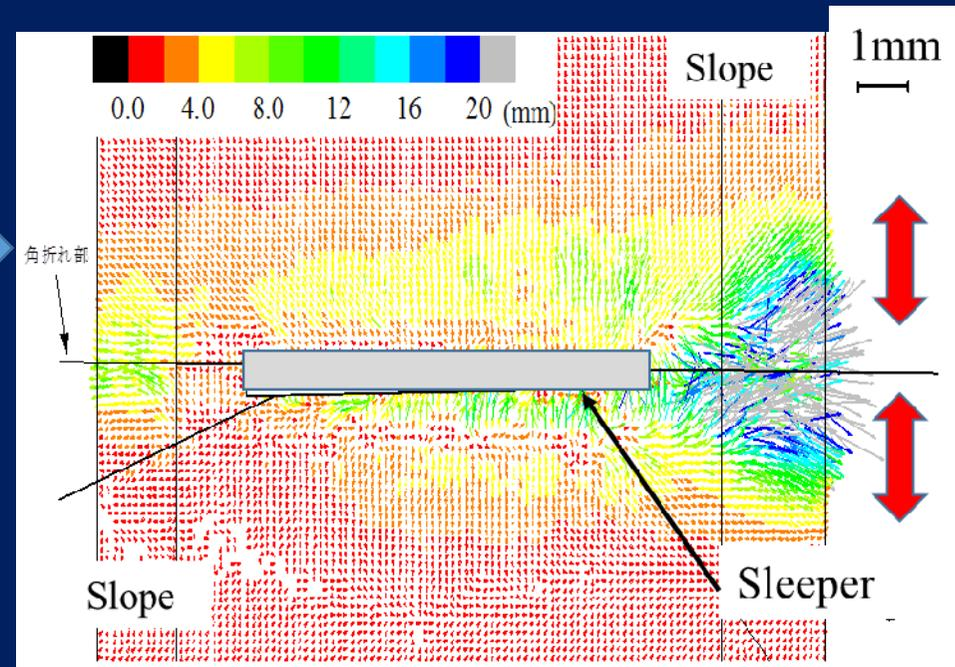
Accumulated displacements after the 20<sup>th</sup> cyclic loading (folding) from PIV
