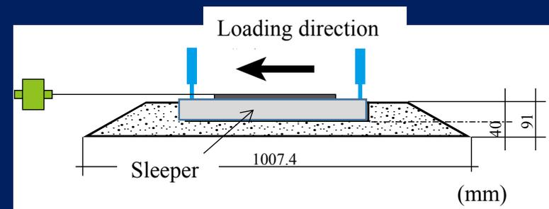
Track panel pull-out test on a 1/5 scale model
