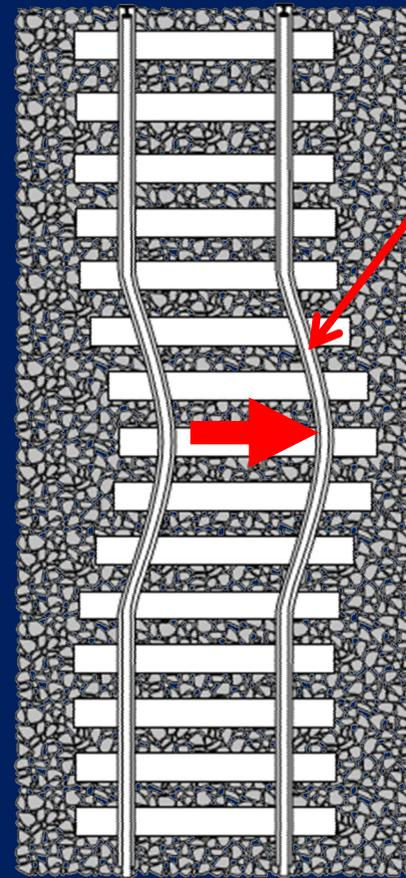
Increase of axial force with the increase of rail temperature
