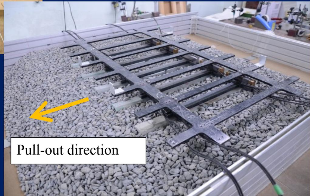
Track panel pull-out tests with 5 sleepers
