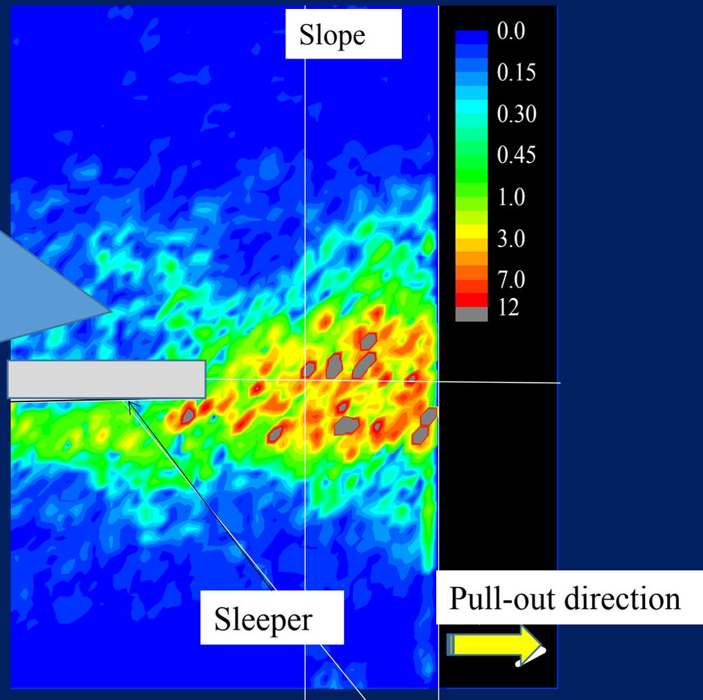
Maximum shear strain distribution near the sleeper end after the 20<sup>th</sup> cyclic loading (folding) from PIV
