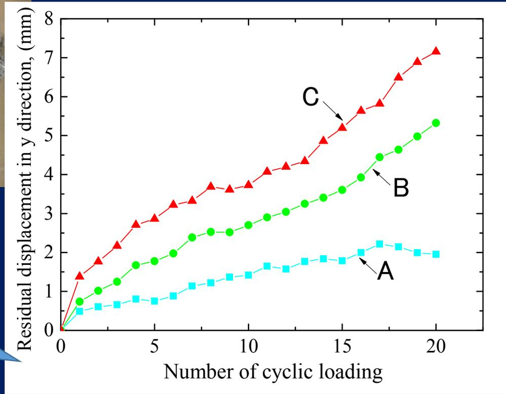
Residual displacements in y direction at points A, B and C near the sleeper side from PIV
