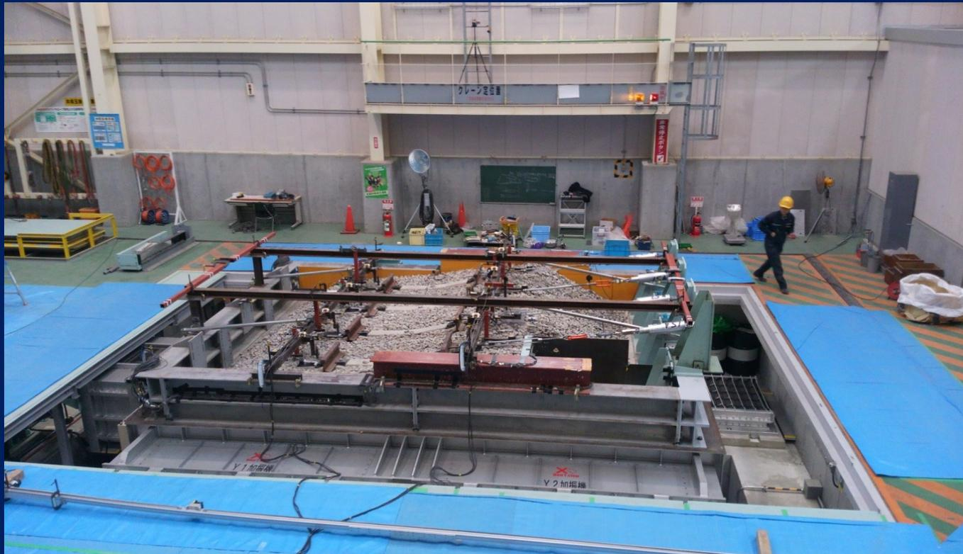
Shaking table tests on a full-scale ballasted track
