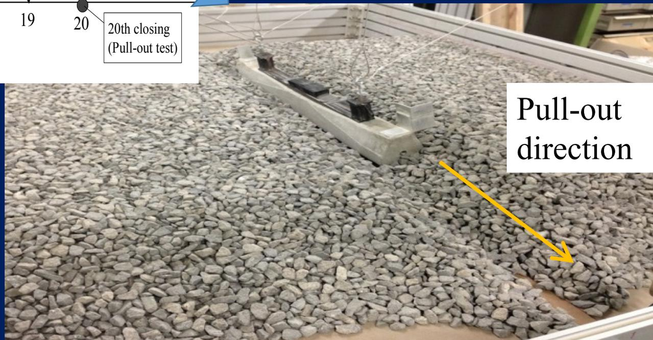
Single sleeper pull-out test at 20th opening
