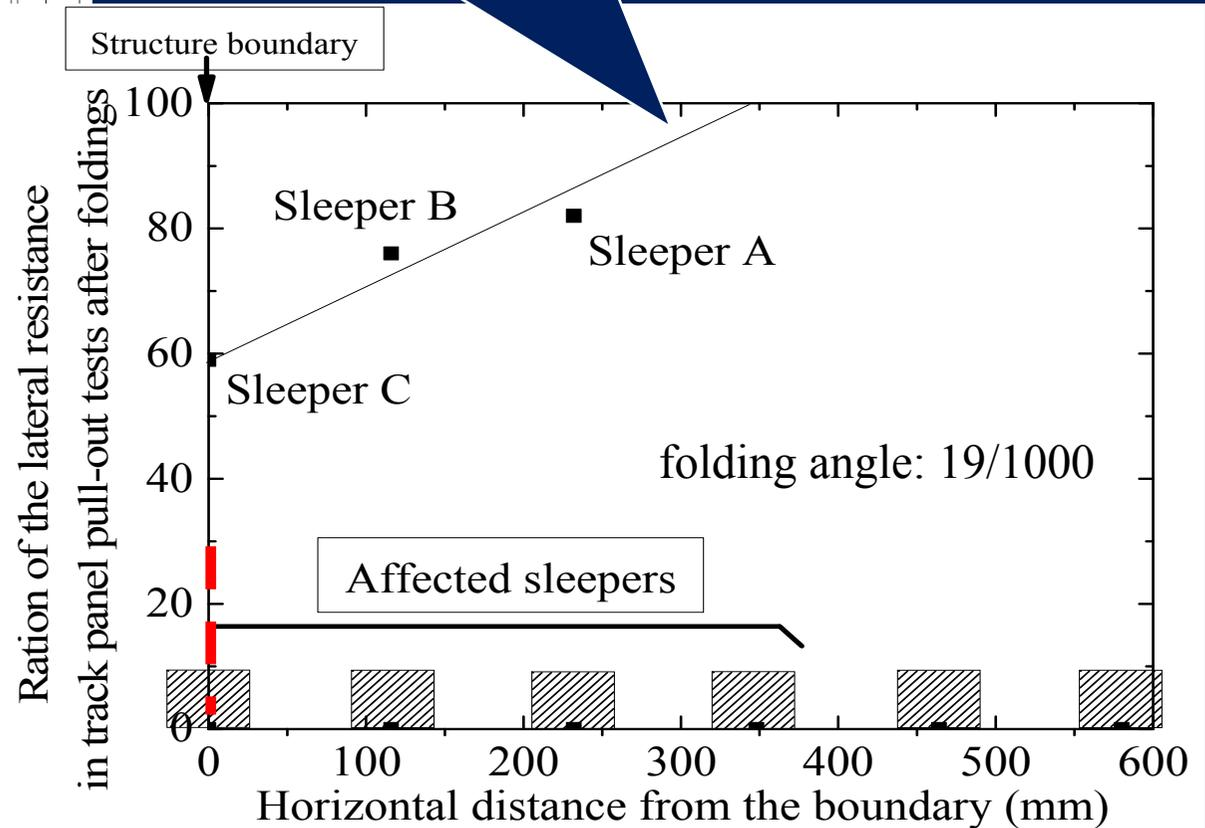
Ratio of lateral resistance of each sleeper before folding to that after folding
