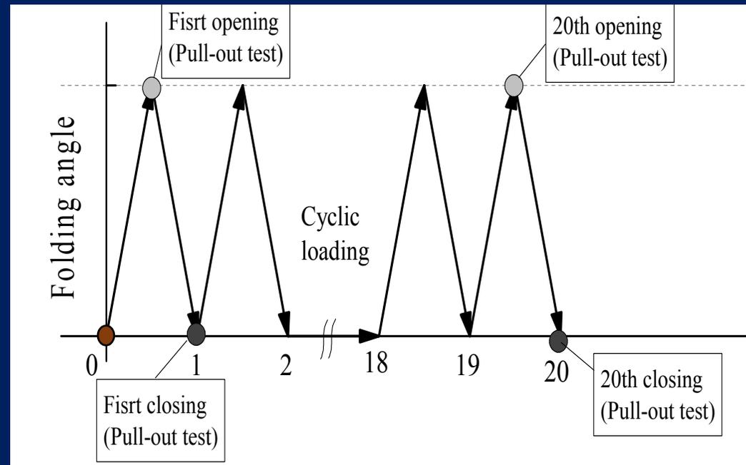
Physical modeling of cyclic loading (folding) in model test and sleeper pull-out tests under opening or closing situation
