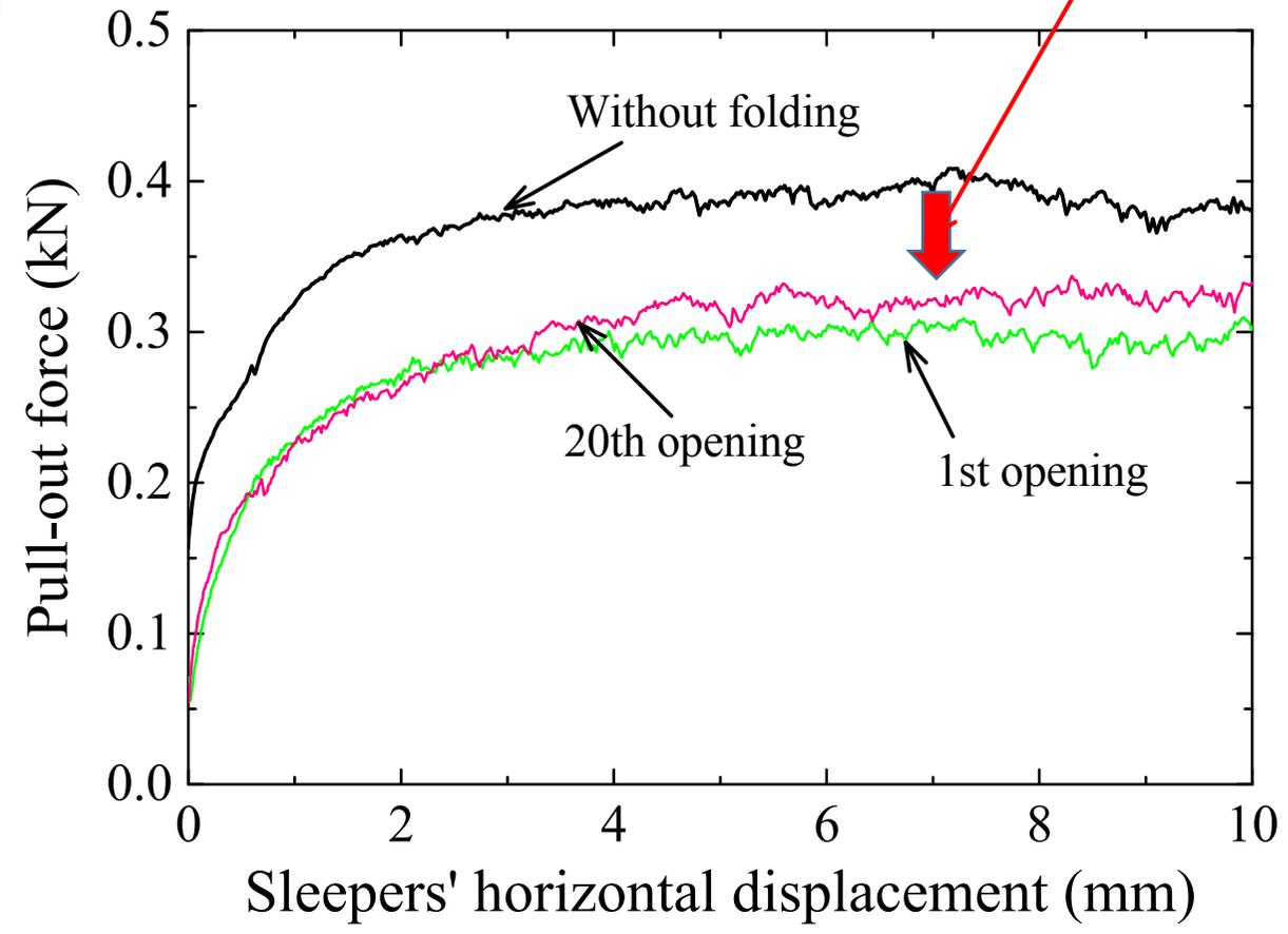
Track panel pull-out test results(folding angle: 19/1000)
