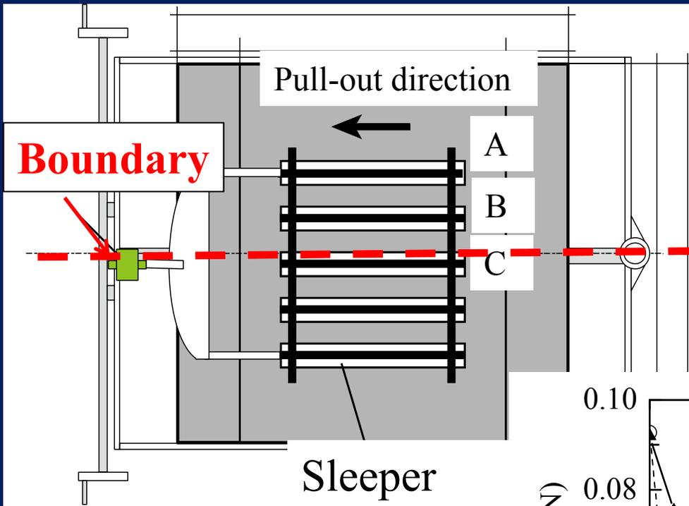
The more away from the structure boundary, reduction of the lateral resistance is less significant.
