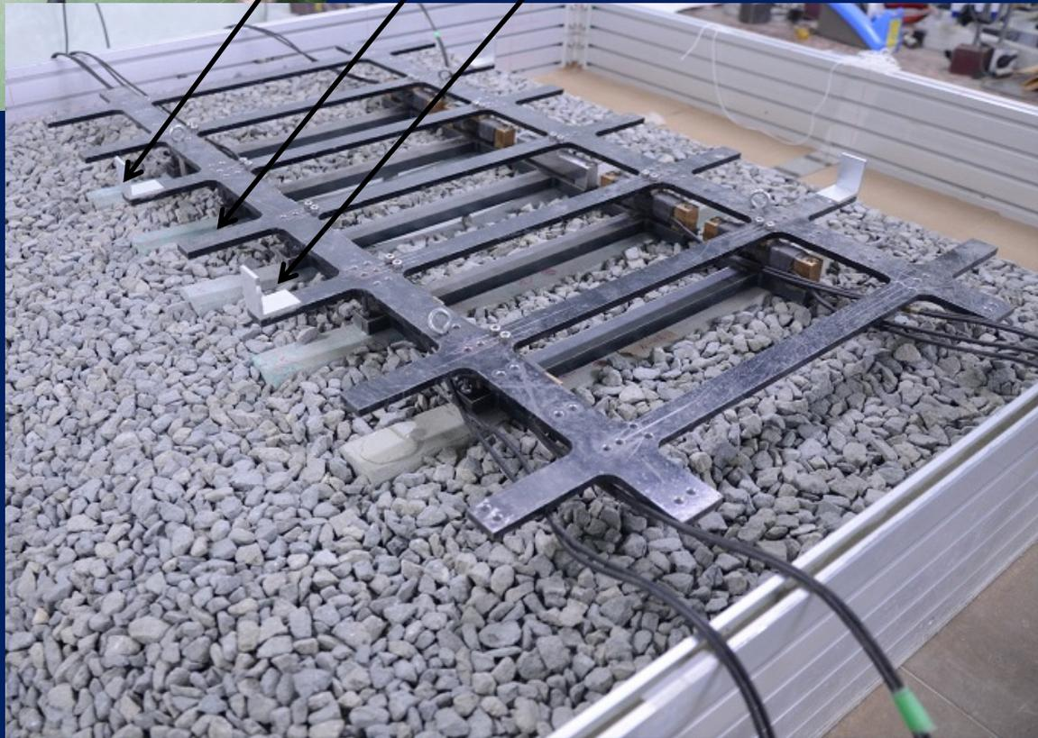
Load cells were installed on the sleepers so that lateral resistance of each sleeper could be measured in the track panel pull-out tests.
