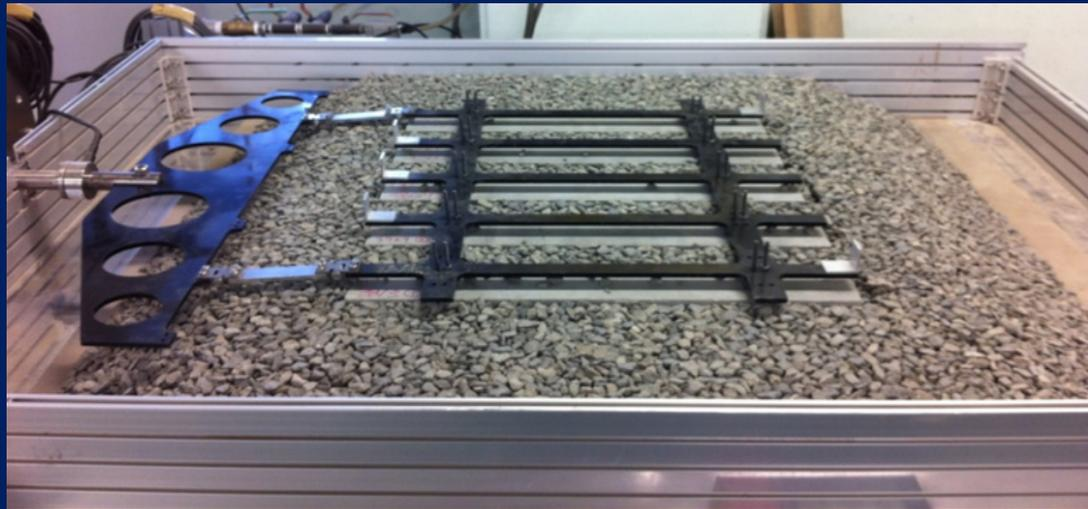
Small scale (1/5 scale) model tests
